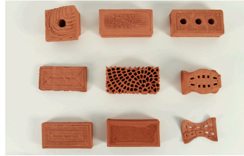
3-Axis extrusion production samples. Brick Geometries , MArch I Thesis, K. Hinz. Photo: K. Hinz, 2016.
