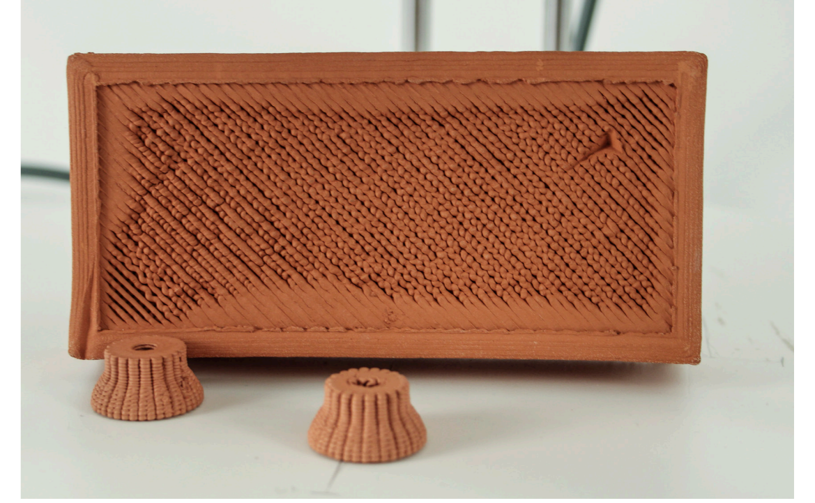
Fully fired sample brick (shown during printing at left) illustrates unique tooling parameters that cause viscous folding in the final extrusion layer. Photo: K. Hinz, 2016.
