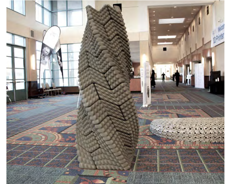
3D Printed "Sand" Masonry, V. San Frantello & R. Rael
